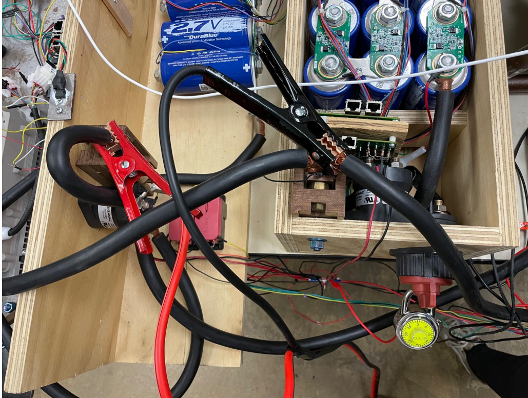
Figure 2. Proper jumper cable connection to capacitors.
